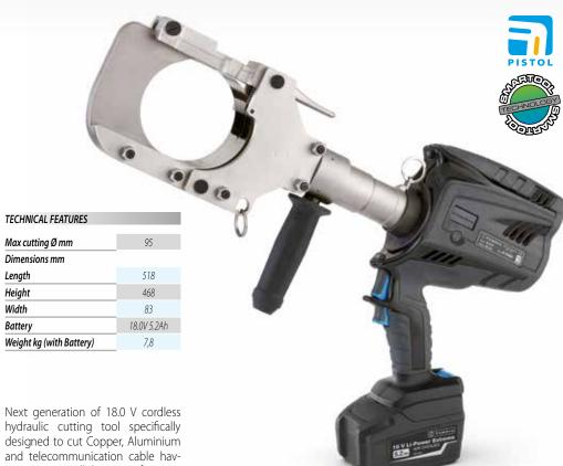
ing a max overall diameter of 95 mm. The blades are manufactured from high strength special Steel, heat treated to ensure a long service life. New Li-lon 18.0V - 5.2Ah batteries offer a higher capacity, while greater cutting speed and cutting force result from a revitalised hydraulic system with double speed action.
