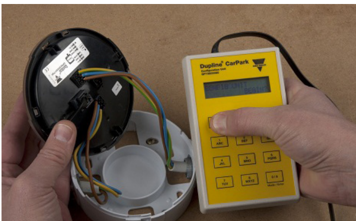
Fig. 40: Sensor and programmer GP7380 0080
