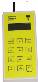
Fig. 23 : Parking guidance test and configuration unit - GP 7380 0080 709
