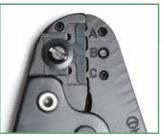
Emergency release lever which, if necessary, opens the crimp jaws before their complete closure.
