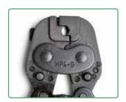
At the end of the crimping the outer surface of the conductor is automatically stamped with the following crimping code:
