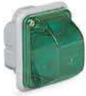
Signalling lamps in thermosetting GRP with E14 lamp holder for flush-mounting IP65
