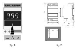
Figure 2 shows the overall dimensions and the panel cut-out.
