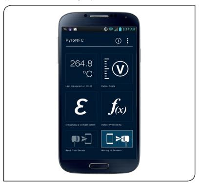
Touch the NFC device against the back of the sensor to read the measured temperature. The reading updates continuously while the phone is touching the sensor.
