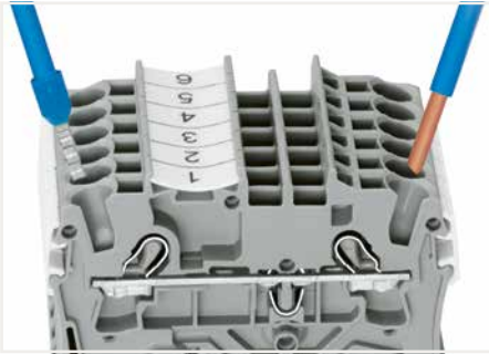
Insert solid and ferruled conductors via push-in termination.
