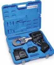
Next generation of 18.0 V cordless hydraulic cutting tool specifically designed to cut Copper, Aluminium and telecommunication cable having a max overall diameter of 65 mm. The blades are manufactured from high strength special Steel, heat treated to ensure a long service life.
