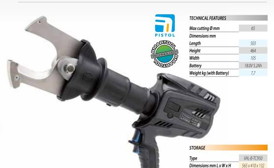
Next generation of 18.0 V cordless hydraulic cutting tool specifically designed to cut Copper, Aluminium and telecommunication cable having a max overall diameter of 65 mm. The blades are manufactured from high strength special Steel, heat treated to ensure a long service life. The open head and the "scissor" movement of the blades facilitate the cutting of running cables.
