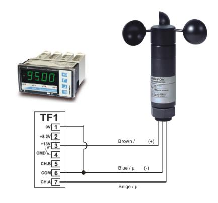
Just feed the supply voltage to the UDM35 controller, it will display the number 0 (zero) on screen.
