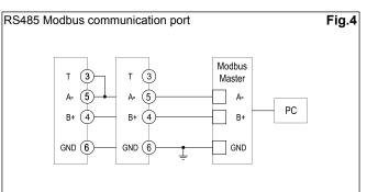
Additional instruments with RS485 are connected in parallel. The serial output must only be terminated on the last network device connecting terminals A- and T. For connections longer than 1000 m use a signal repeater. Maximum 247 transceivers on the same bus.
