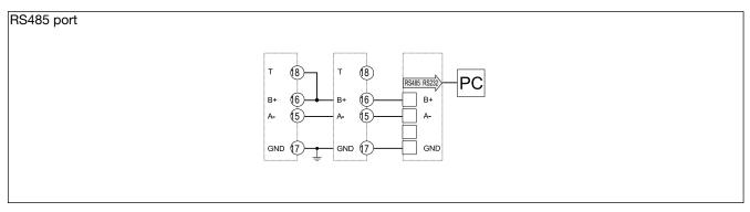
**RS485 NOTE:** additional devices provided with RS485 are connected as per the picture above. The termination of the serial output is carried out only on the last instrument of the network, by means of a jumper between (B+) and (T).
