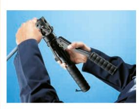
The operator can advance the dies using only one hand, leaving the other hand free to position the connector.
