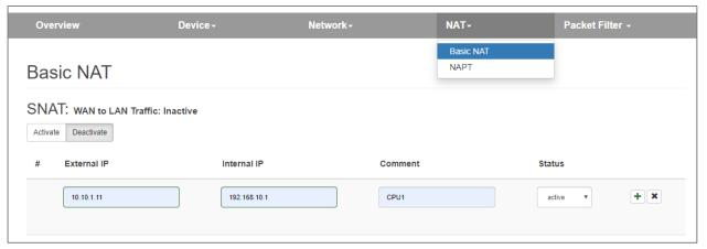
The "External IP" is the IP address under which the network participant of the machine becomes visible in the production network (WAN). The "Internal IP" is the IP address of the network participant in the machine (LAN). Any text can be entered as a comment.
