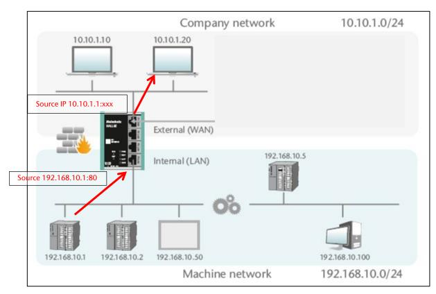
The option "NAPT: Active" thus enables communication of devices from the LAN with devices in the WAN. WALL IE thereby acts as a gateway to administer the implementation to the IP addresses of the WAN network and looks after the assignment of the response.
