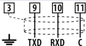
Connect any shield of the cable to terminal 3.
