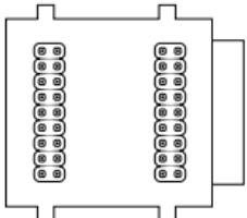
Bus connector to be lodged in the hollow of the DIN rail to connect any I/O module to the PL500. For the mounting sequence see paragraph [2.2](#).
