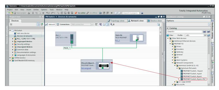
By calling up the properties in the device view, you must assign the PROFINET-Switch a unique PROFINET name in the project and check the IP address for plausibility.
