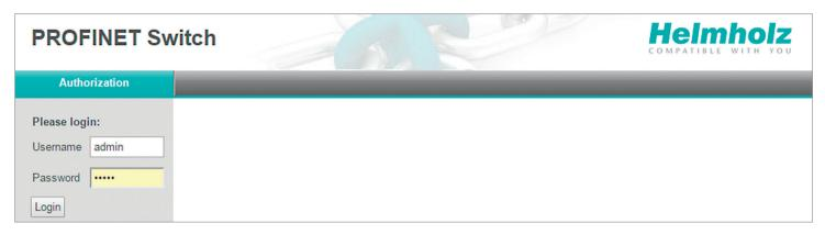
When the web interface is first called up, the password of the "admin" user is the serial number of the device. The serial number is printed on the right housing side part (e.g. "50001234"). It is absolutely necessary to assign a new password following the first login:
