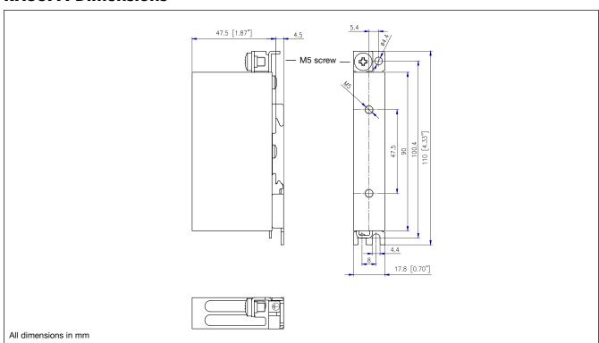
Note: M5 PE screw not provided with SSR. Maximum mounting torque 1.5Nm (13.3 in-lb). PE connection required when product is intended to be used in Class 1 applications according to EN/IEC 61140.
