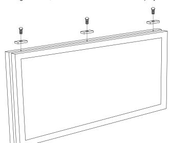
The display must be mounted by using the included hammer nuts.
