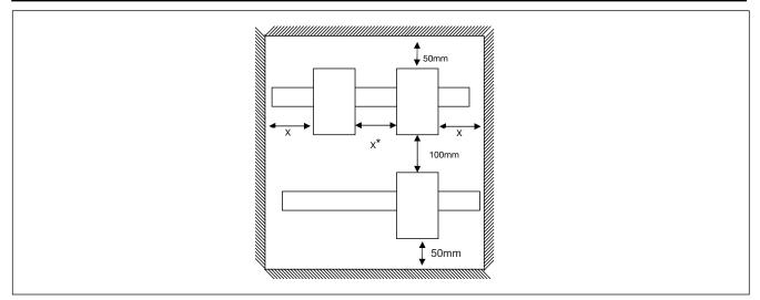
\* Refer to Current Derating vs spacing curves. Spacing between SSR and panel walls should be >5mm.
