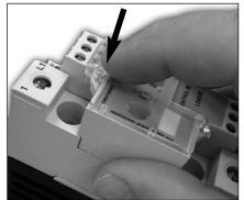
2: Close the cover by clipping to the top loop of the RGx1P control module
