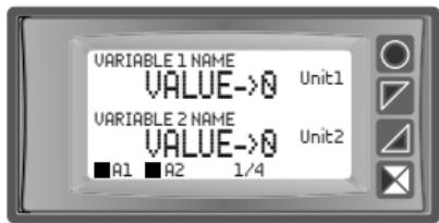
Shows the value of a variable by means of alphanumerical strings instead of the corresponding numerical value. This is possible for variable values between 0 and 4. A text string 8 characters long can be set for each of these values. For values lower than 0 and higher than 4, the variable is displayed in the traditional numerical format.
