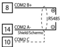
For connection to a Modbus master device
