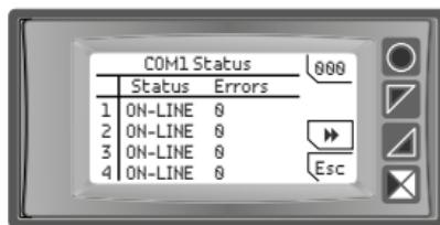
It indicates the current status of the variable (ON-LINE, OFF-LINE) and the number of communication errors or timeouts since the instrument was switched on.
