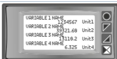
Shows the value of the first four variables enabled with relative description, unit of measurement and status of the alarm relays. The figure represents the display of "4 val. per page" setting in "Display -> View" parameter.
