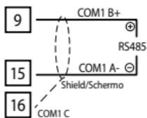
For connection to Modbus slave devices
