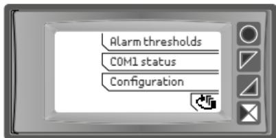
The keys are multifunction: the instrument shows the meaning of the various buttons on the display near the relative key. If there is no text near the key, press any button to display it. Some menus are only displayed if activated.
