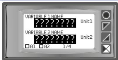
Represents the typical display of variables in offline mode. If the STR571 display cannot establish the connection with the slave of the variable, and therefore cannot read/write the relative value, the numerical display is replaced by flashing question marks.
