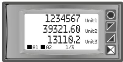
Shows the value of the first three variables enabled, in **expanded view mode**. This mode, which can only be enabled when viewing 3 or 4 variables per page, displays the values of the variables with a larger character than that normally used for this representation, without viewing the description of the variables and only leaving the unit of measurement. This mode is enabled by setting the description of the relative variables as a sequence of spaces (zero description).
