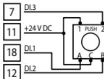
The drawing shows how to connect the encoder from the optional panel to browse and edit the values of the variables. (Code 5300.55.001)
