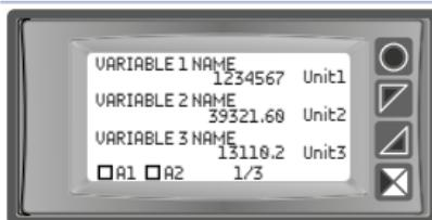
Shows the value of the first three variables enabled with relative description, unit of measurement and status of the alarm relays. The figure represents the display of "3 val. per page" setting in "Display -> View" parameter.
