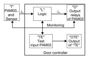
Functional verification procedure for the test input safety-related part of a control system (SRP/CS)
