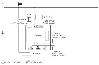
Fig. 3 Single-phase system with neutral (2-wire)
