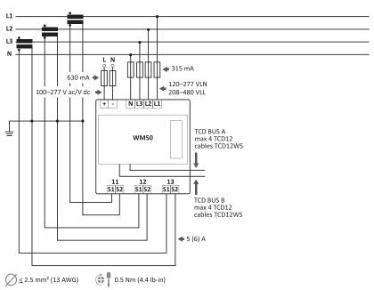
Fig. 1 Three-phase system with neutral (4-wire).
