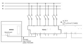
Fig. 13 Two-phase system with neutral (3-wire)
