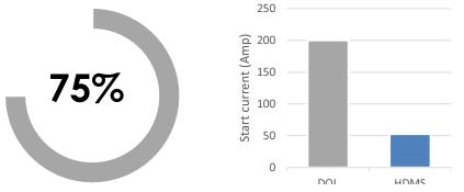
Actual current reduction vs DOL for borehole pump
