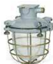
UNAV 2139 large light fixture in marine grey painted brass with stainless steel protective cage with UNAV 1948 cable gland 230V IP66
