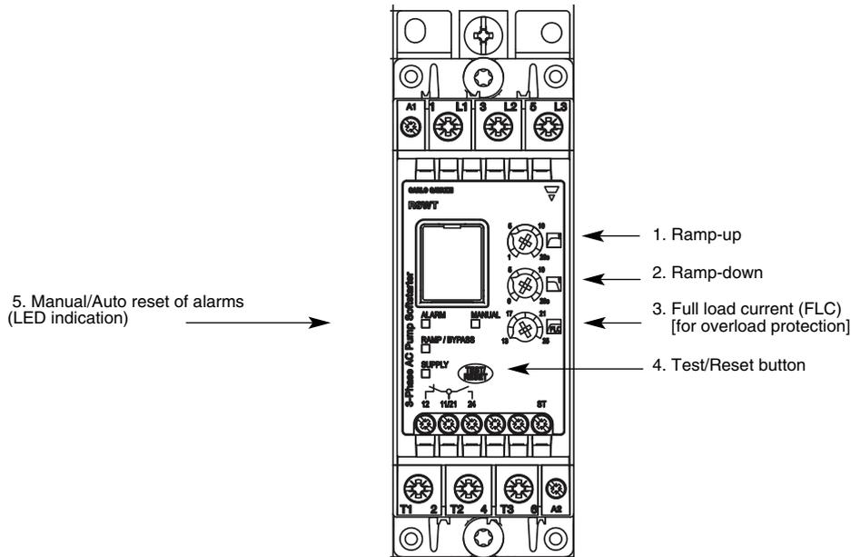
The RSWT...V10/ V110/ V111 soft starter series features 3-knob settings and an additional push button to test the overload protection, reset the alarms and for setting the alarm recovery to Manual or Auto.
