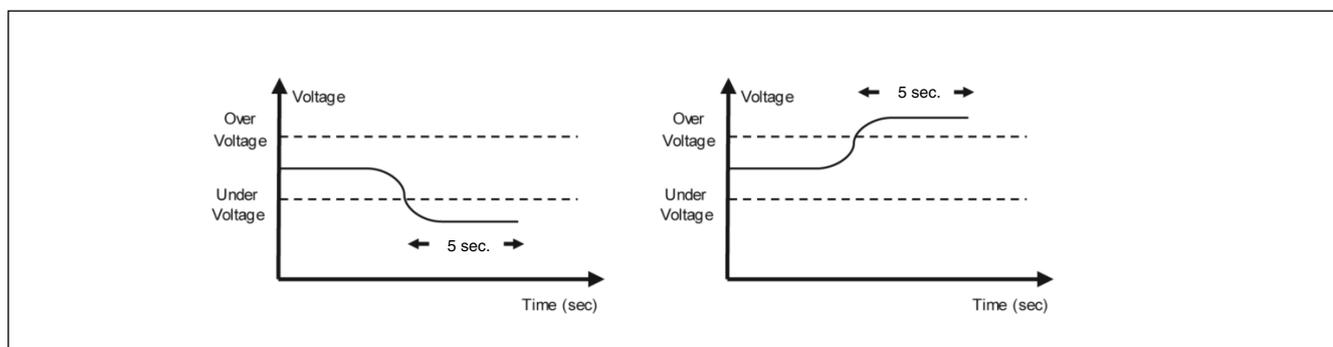
At every power-up the RSWT automatically detects the supply voltage level and determines whether it is working on a 220, 400, 480\* or 600\* V supply. The under- or over- voltage alarm level is then set at a level of -20% and + 20% (from the measured supply voltage level) respectively. If the supply voltage level is out of these limits for more than 5 seconds then the line voltage out of range alarm will be triggered.
