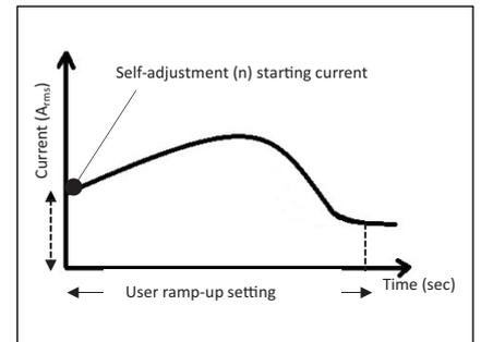
**Start n:** For the nth start, the RSWT algorithm will keep the ramp-time as close as possible to the user set-ramp time. The self-adjusting algorithm will remain active at every start to make sure that the RSWT adapts the starting parameters to any load changes.
