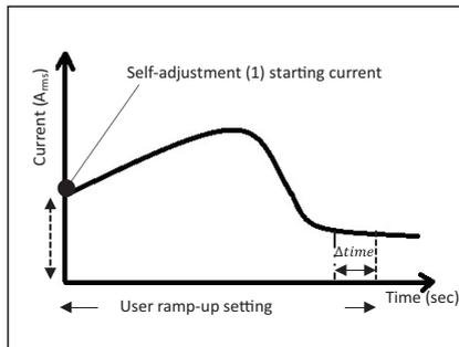
**Start 2:** During the 2nd start, the RSWT will start with the “self-learned” start parameters (from the previous start) to reduce the difference between the user-set ramp-time vs the actual ramp-time measured by the RSWT ( $\Delta$  time).
