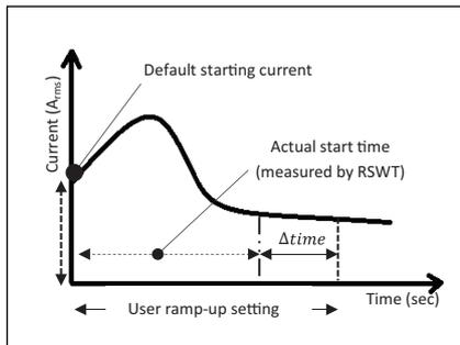
**Start 1:** RSWT starts from default starting voltage/torque (internal) value. The pump start time can be shorter/longer than user ramp-up setting.
